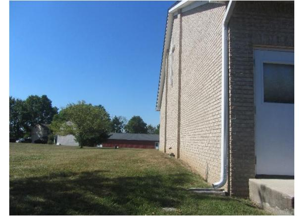
Parking spots in front of the building can be replaced with porous asphalt to capture and infiltrate stormwater. Installing a rain garden adjacent to the building can capture, treat, and infiltrate roof runoff. A preliminary soil assessment suggests that the soils have suitable drainage characteristics for green infrastructure.
